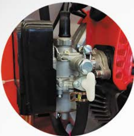
Float Type Carburetor
